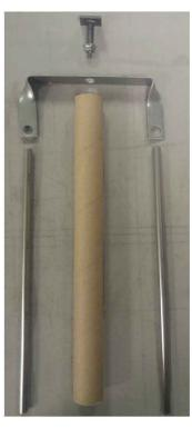
1"x1" Mild Steel plate welded 304 S.S. Stud 304 S.S. Channel Yoke 304 S.S. Tubes (2) Flanged Nut Access Tube
